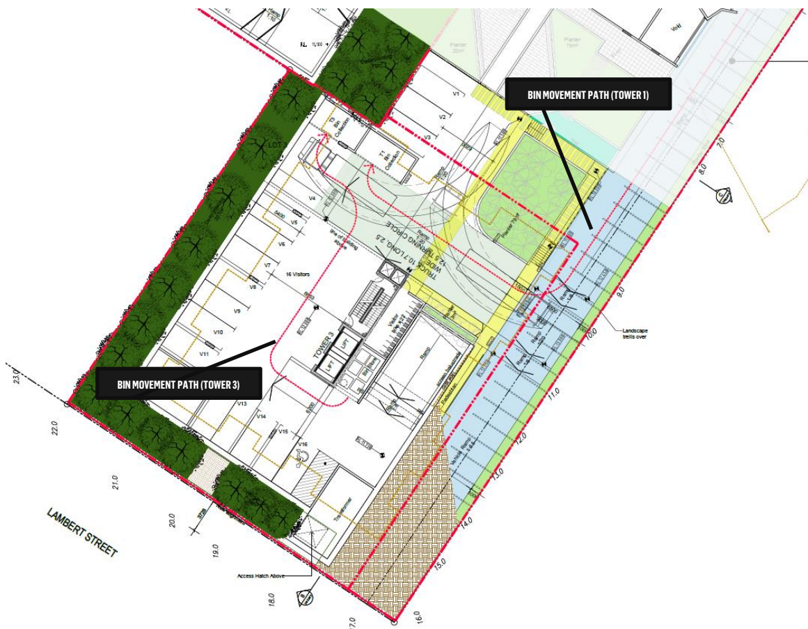
Figure 7 - Swept Paths for Tower 3 Refuse Vehicle Collection
